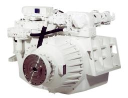
Horizontal offset, remote mount marine transmission.
